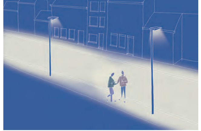
- Optic LensoFlex®2 "Residential street" 5103 - For M4 classification according to CIE 115
