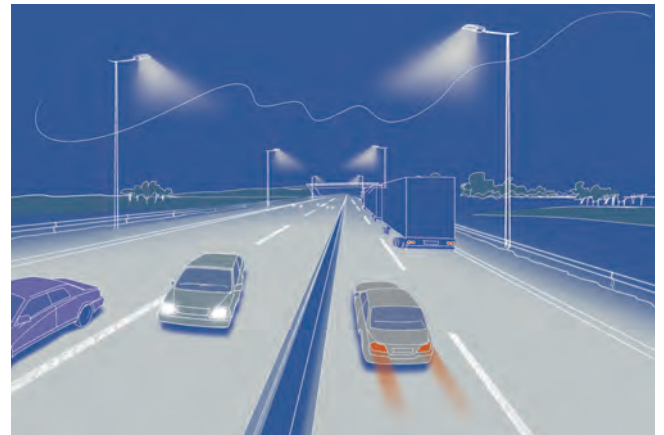
- Optic LensoFlex®2 "Motorway" 5102 - For M3 classification according to CIE 115
